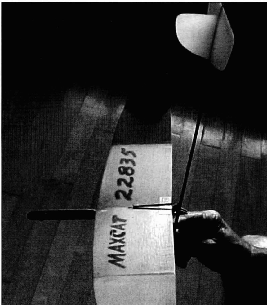
This view from above shows the attractive wing outline, borrowed from Stan Buddenbohm's Apex design. Tim likes the 6-panel layout: He believes it enhances thermal stability. (Tim Batiuk photos)
